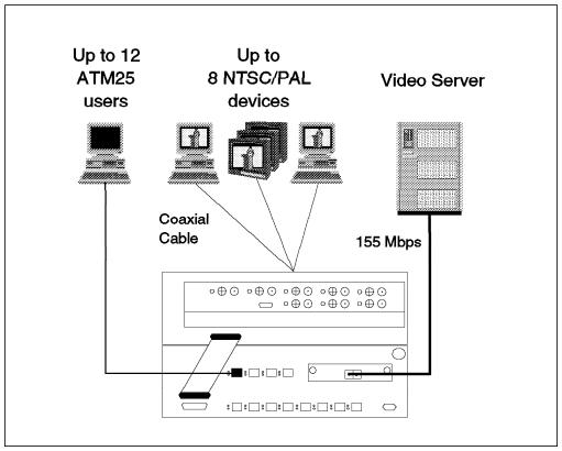
Figure 20. Video Distribution Module Workgroup Configuration
